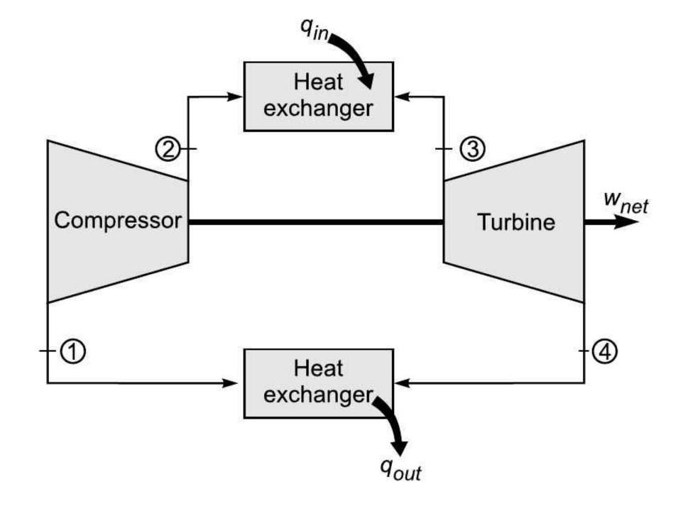
The Brayton cycle consists of four internally reversible processes:
