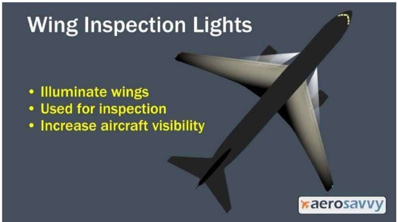
Fig no. 1.7: Wing Inspection lights
