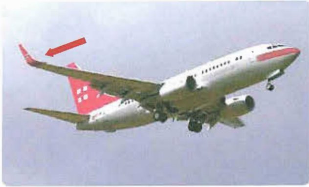
Figure 1-38. A winglet reduces aerodynamic drag caused by air spilling off of the wing tip.
