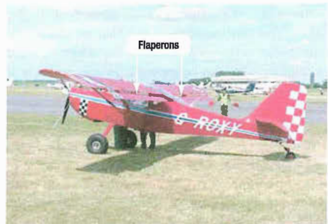
Figure 1-27. Flaperons on a Skystar Kitfox MK 7.
