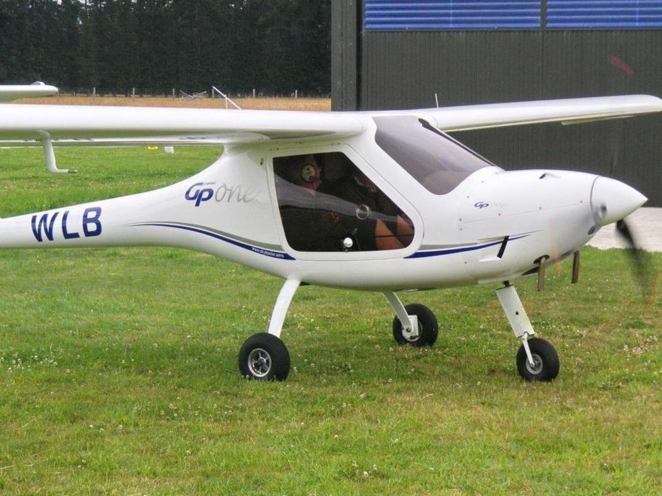
The most commonly used landing gear arrangement is the tricycle-type landing gear.
