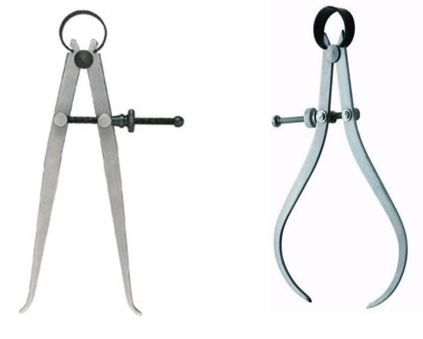
They are usually of two types- inside and outside caliper. They are used to measure internal and external size (for e.g. diameter) of an object. It requires external scale to compare the measured value.
