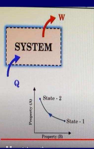
During a Process 1-2, Heat added to the system is Q. Work done by the system is W.  $Q_{1-2} = \Delta E + W_{1-2}$  $Q_{1-2} = E_2 - E_1 + W_{1-2}$  $Q_{1-2} = (U_2 + KE_2 + PE_2) - (U_1 + KE_1 + PE_1) + W_{1-2}$  $Q_{1-2} = U_2 - U_1 + W_{1-2}$  $Q_{1-2} = \Delta U + W_{1-2}$ Theater mode (t) Applicable for Stationary Closed
