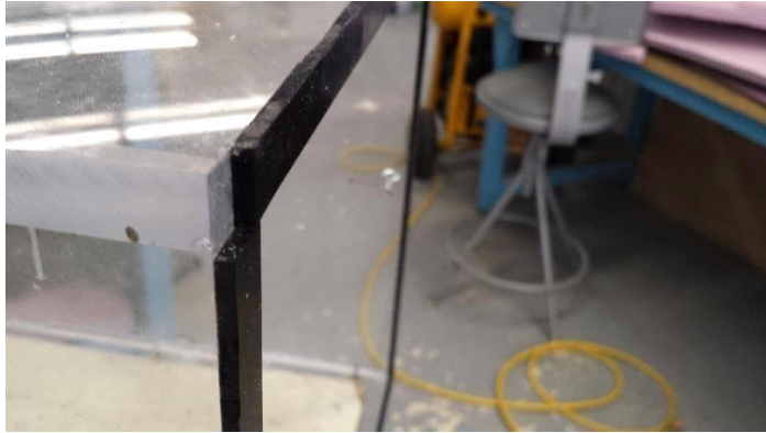
Rubber gasket used to line test section connecting edges fig 3.10
