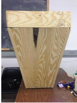
Completed contraction section, side View fig3.6
