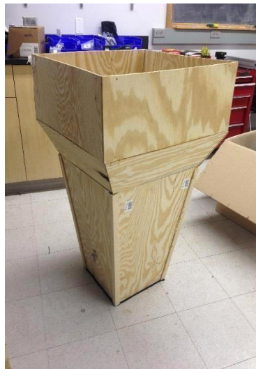
Completed wind tunnel diffusing section fig 3.11
