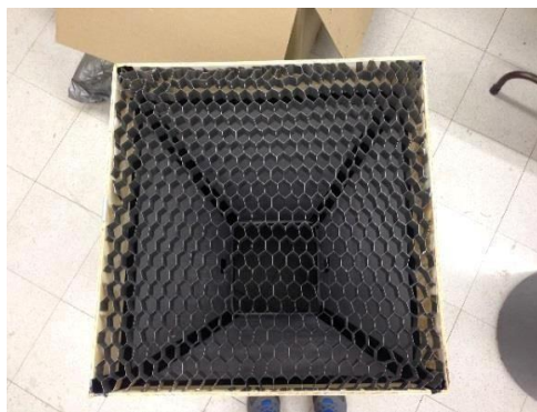
Completed contraction section, aerial view
