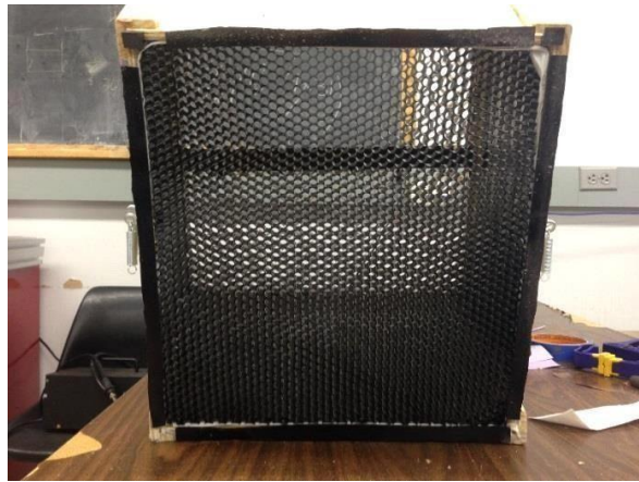
Second honeycomb structure, located at end of contraction section
