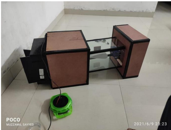
Fully assembled wind tunnel structure fig 3.13
