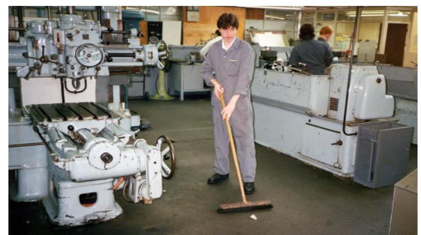
• Chips should be removed from the table or bed of a machine Because metal chips have sharp edges, which cut and penetrate skin, chips should *never* be handled. Machines can be kept clear of chips.by periodically sweeping (or brushing) them away.
